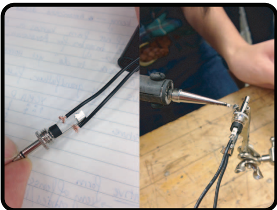
Step 7 (we did this already): Wrap wire around audio jack and solder before replacing cap
