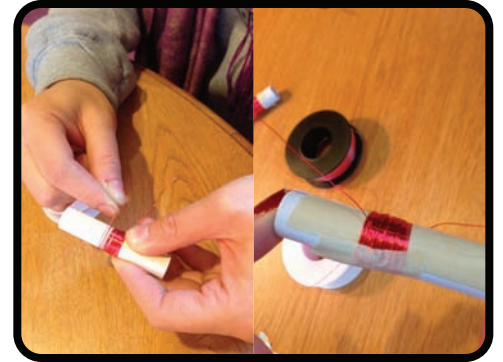
Step 3: Leaving a bit for the ends, wrap the magnet wire 50 times around the paper tube with magnet
