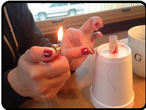
Step 4: Burn magnet wire ends
