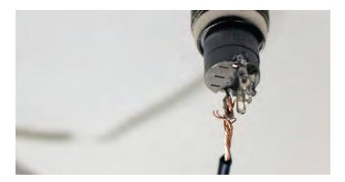
6. Now that there are several connects, use the multimeter to test if the connections are strong and will carry a current. Put one tip of the multimeter on one end of your circuit, and another top at the other end. If the needle on the multimeter moves, the connections are good. If it does not, check for loose solder or wires.
