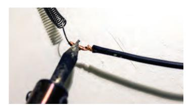
7. Feed one end of the thermostat switch into another prong of the button switch. Make a hook connection and solder it.
